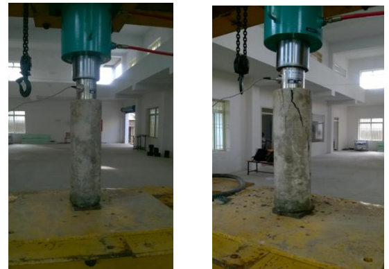
Fig.No.7 Testing of column
