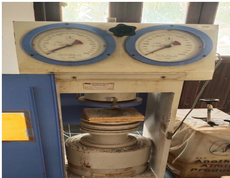
Figure 1: Brick under compression testing machine
