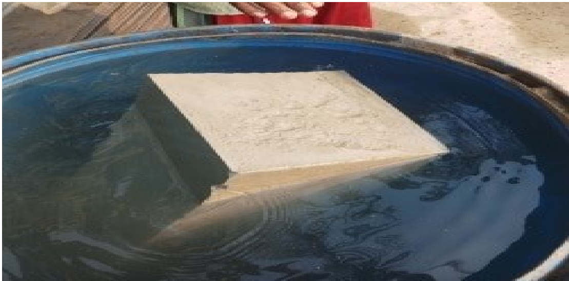
Figure 2: Brick under Water absorption Test
