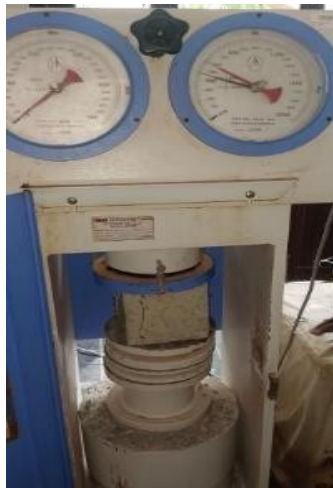
Figure 1: Cube under compression testing machine
