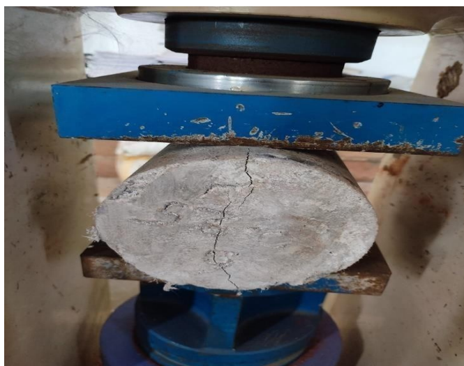
Figure 3: Cylinder under split tensile testing machine
