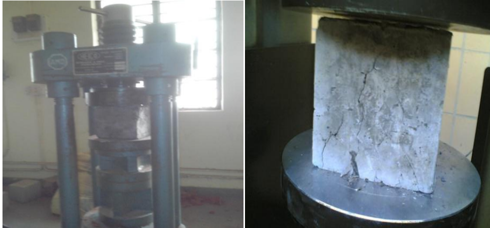
Figure 5 Testing of cement concrete cubes during and after test
