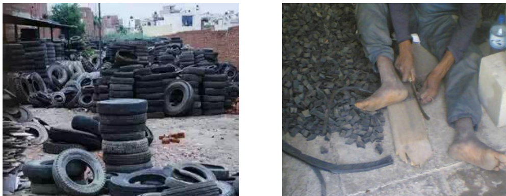
Figure 1 Stockpile of waste tyres and process of rubber aggregates preparation manually
