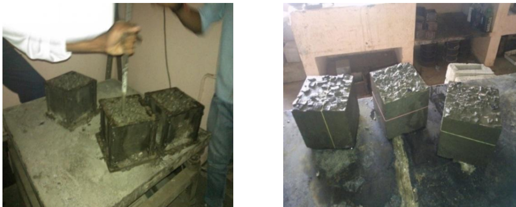
Figure 4 Casting of concrete mix using table vibrator and its air curing process
