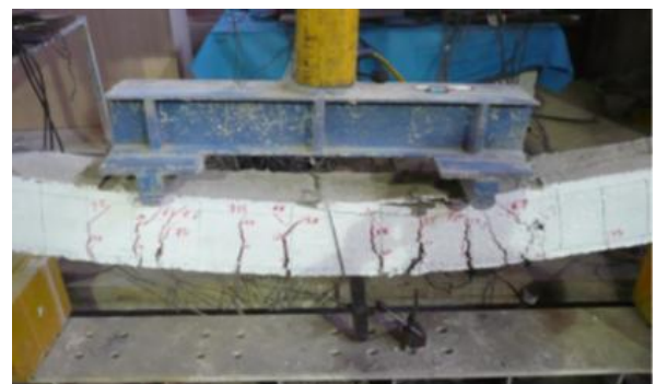
Fig. 7. Test of RC beam
