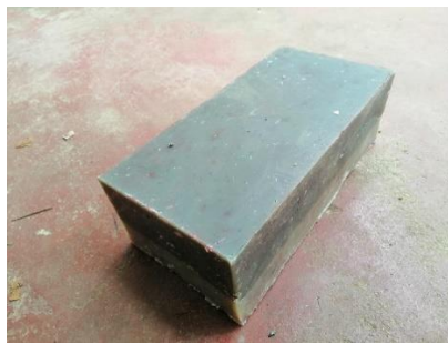
Fig6: Paver block after demoulding
