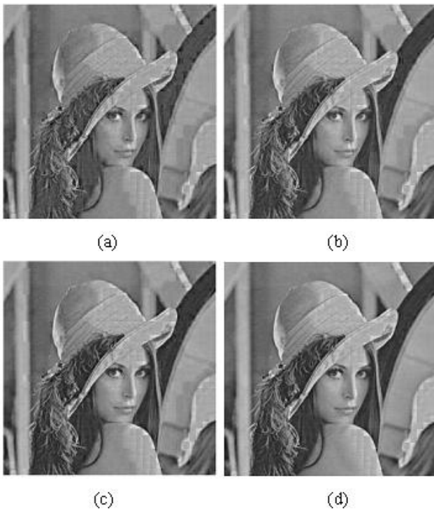
Fig.3 Results using Improved DCT with LBG algorithm for different Codebook Size (a) codebook size=128,(b) codebook size =256,(c) codebook size =512,(d) codebook size =1024
