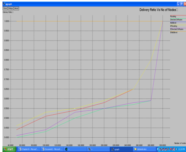
Figure 3 Performance Graph for Delivery Ratio Vs Number of Nodes Table 1 Simulation scenario
