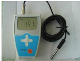
Fig 4) Temperature data logger
