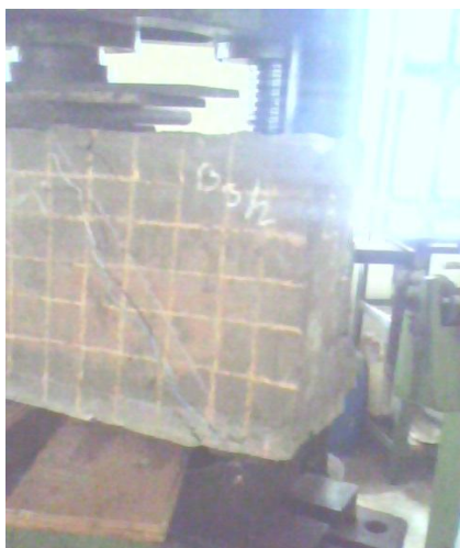
Image 7 Deep beam testing
