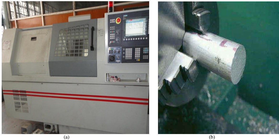
Figure 1 Photographic view of (a) CNC facing and (b) experimental set-up
