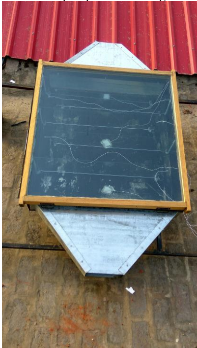
Fig.8 Solar air collector with multi-pass arrangement made from transparent glass.
