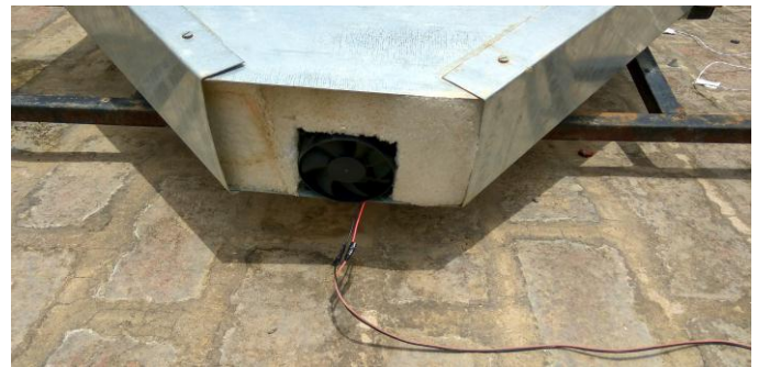
Fig.11 Variable speed 12V DC Fan.
