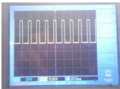
Fig.18 Output pulse of driver circuit with shoot through(12V)
