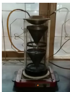
Figure 2. RAP Extraction Testing
