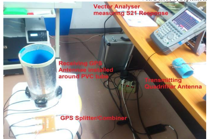
Figure 6. Measurement of S21 radiation pattern using R&S ZVH-8
