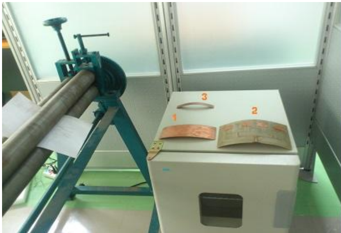
Figure 9. FR-4 substrate no.1 and no.2 of 1.6mm thick with their maximum curvatures, and the easier-to-bend substrate no.3 of 0.8mm thick
