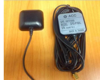
Figure 3. Active GPS antenna with 28dB gain (cable loss not included)
