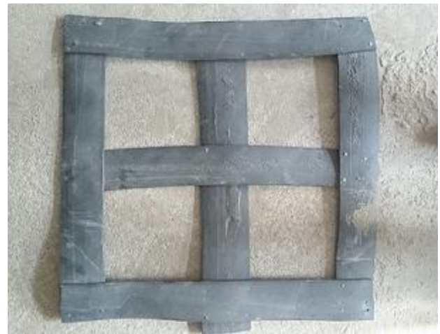
Fig.2.1 Square Rubber Grid used in the Test
