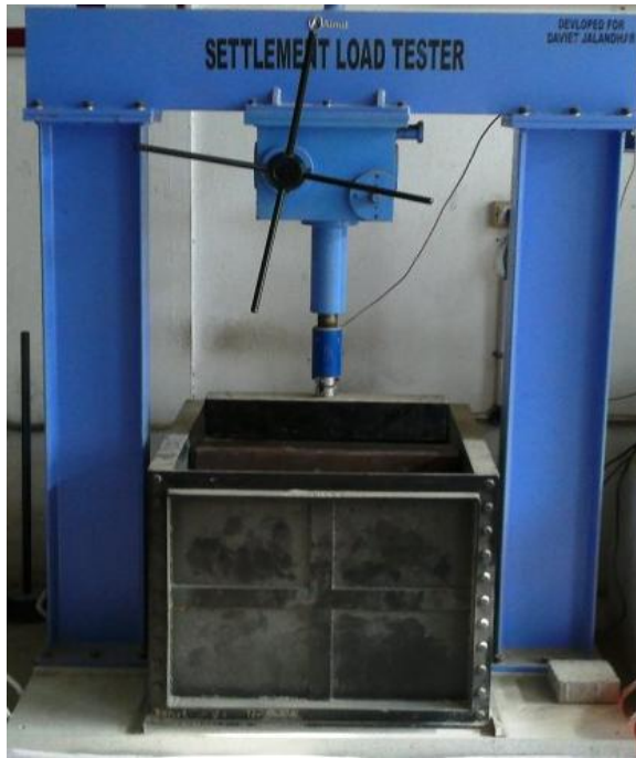
Fig.2.2 Settlement Load Tester
