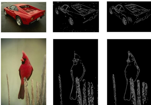
Figure III-9 Output of the Canny edge detector compared with the output of the sobel (right column) edge detection with pre-processing
