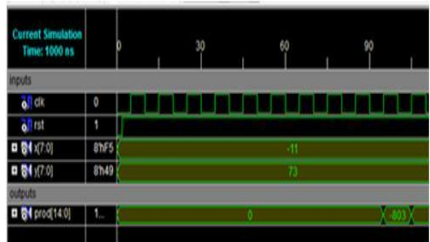
Fig: Simulation results of 8 x 8 signed multiplication using CLA.
