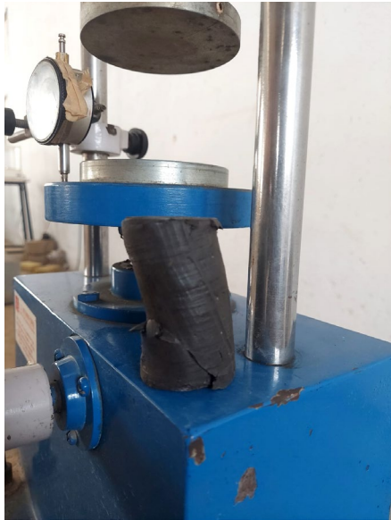
Fig 10. UCS test in lab
