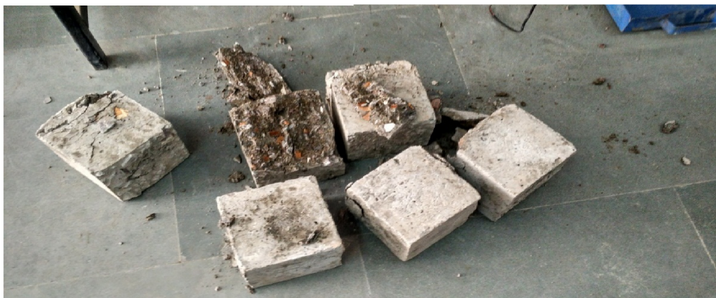
Figure 19: FAILED SPECIMEN AFTER COMPRESSIVE STRENGTH TEST
