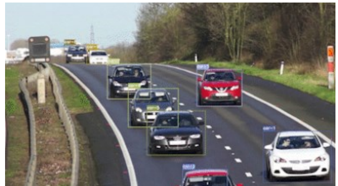
Fig. 2. Illustration of vehicle detection, from video frame capture to bounding box generation
