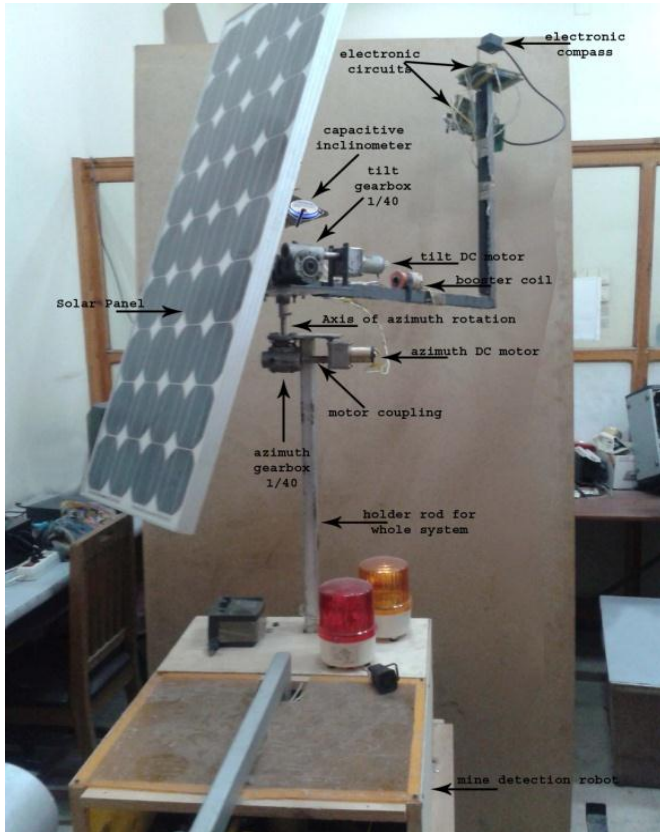
Fig.10. (a) Electronic control circuit (b) Practical tracking prototype system installed on the robot,
