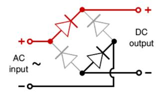
output: full-wave varying DC: (using the entire AC wave):
