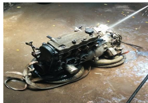
No. 5 – Engine Cleaning and Painting
