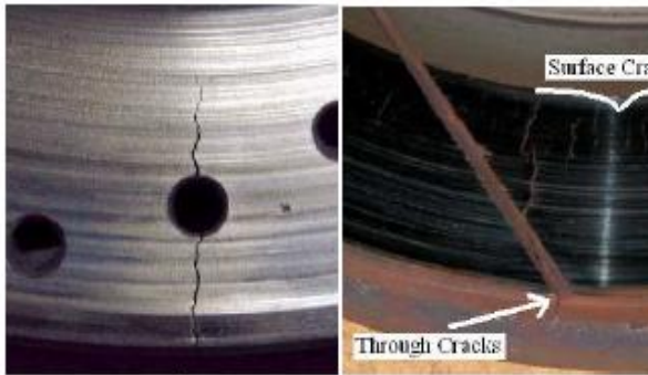
Figure 9 : Brake disc cracking
