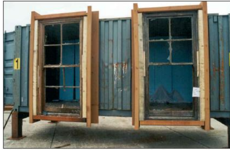
The effects of blast damage can be clearly seen on these windows at a UK explosives research facility.
