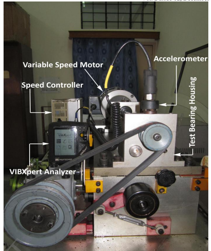
Fig.3 Figure showing Spectra Quest Fault Simulator Setup and PRÜFTECHNIK VIBXpert 2-channel FFT data collector and signal analyser
