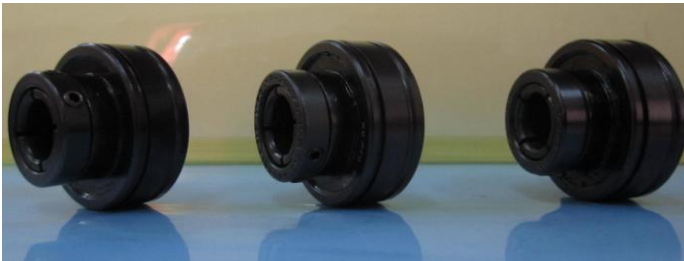
Fig.2 Photograph of MB ER-10K bearings used in experiment
