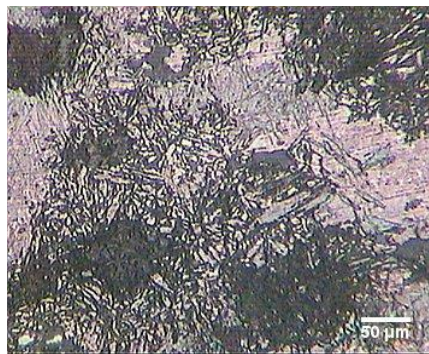
Fig 8(c) Forged Preform at Intermittent Height Strain at 400 X.
