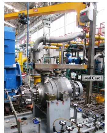
Fig.8. Experimental setup for application of moment M_{yc}
