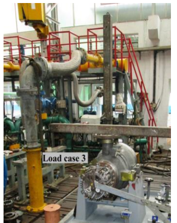
Fig.9. Experimental setup for application of moment M_{zc}
