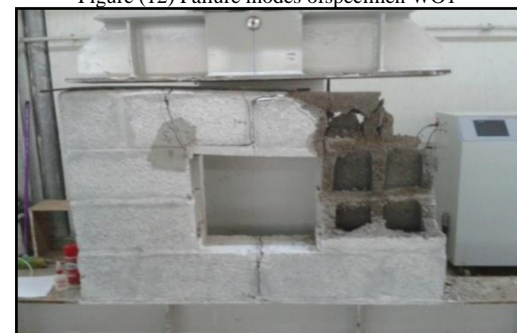
Figure (13) Failure modes of specimen WO2
