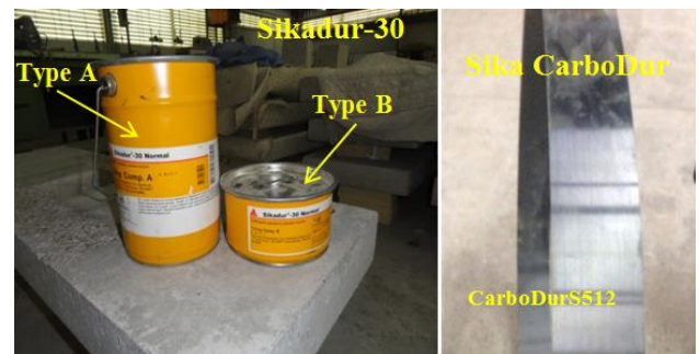
Figure (3) Manufactured forms of CFRP materials
