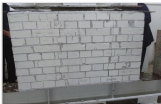
Figure (10) Failure modes of specimen WS1
