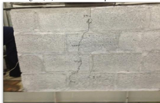
Figure (11) Failure modes of specimen WS2
