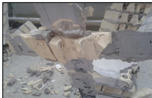
Figure (12) Failure modes of specimen WO1
