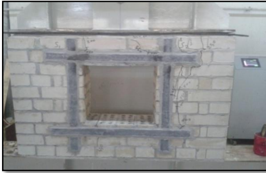
Figure (14) Failure modes of specimen WC1
