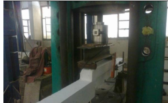
Fig. 2. Test setup for experimental tested beam
