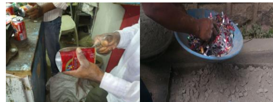
Plate 1: Beverage Tins as Fiber reinforcement.
