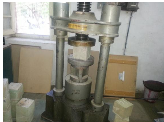
Plate 4 Testing of Cube Specimens
