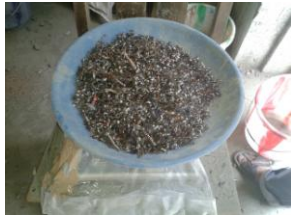
Plate 2 Mild Steel Lathe Waste
