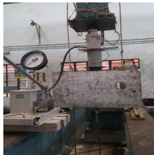
Plate 8: Loading setup of deep beams
