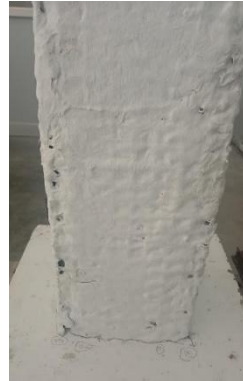
Fig 9 Crack patterns of conventional column Fig 10 Joint failure of retrofitted column
