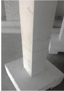
Fig 9 Crack patterns of conventional column Fig 10 Joint failure of retrofitted column
