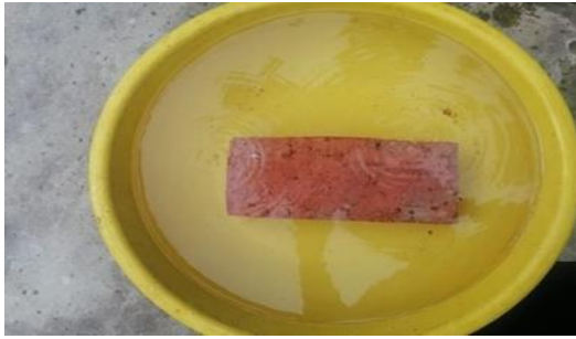
Fig 3.4 Brick immersed in water for absorption test
