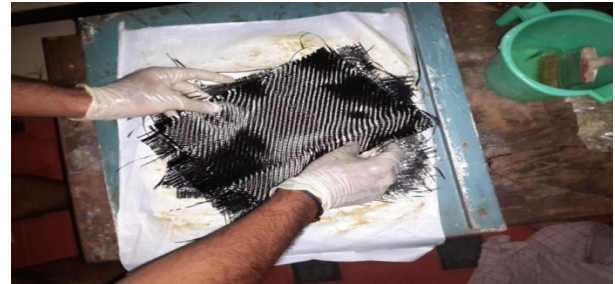
Fig 4. By using hand layup process fabricating the composite
