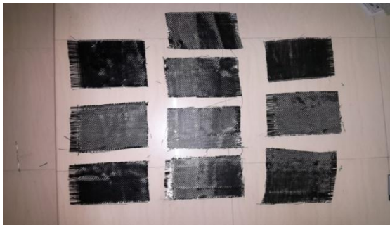
Fig 3. Cut the woven fabric of carbon fiber into 10 pieces of dimension 250mm*200mm
