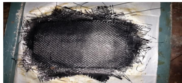
Fig 5. 10 layers of carbon fiber cloth with +30 ply orientation
