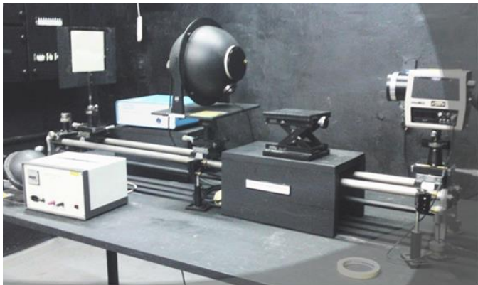
Fig.2 Luminance Measurement setup at NPL, Delhi.
