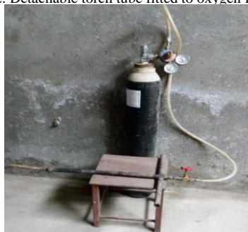
Figure 3: Oxy-iron torch assembly
