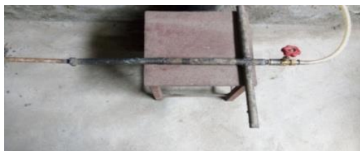
Figure 2: Detachable torch tube fitted to oxygen flow pipe
