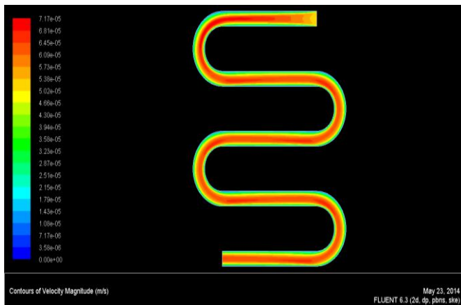
Fig.5.2 Velocity contours of exchanger.
