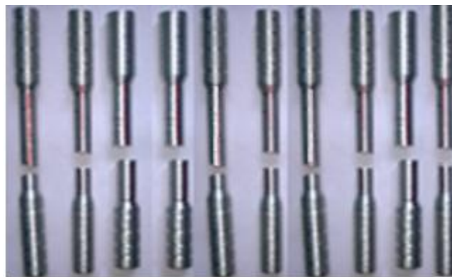
Fig. 9. Tensile specimens after the test
