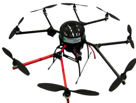
Figure:1. Octocopter (structural inspection flying robot for NDT)
