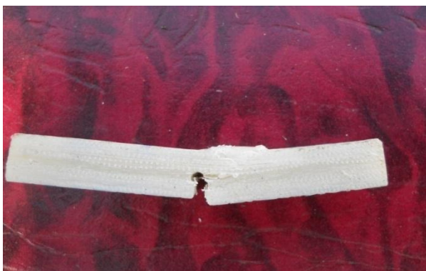
(c) Key hole Notch after delamination
