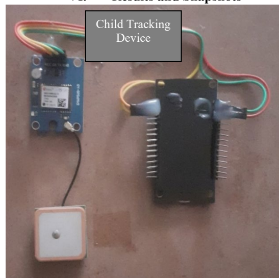
Figure 3: IoT Device for Child Tracking
