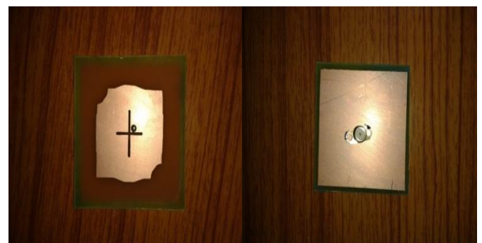
Figure 1 Geometry of single-feed cross slot loaded micro-strip patch antenna: (a) top view and (b) bottom view
