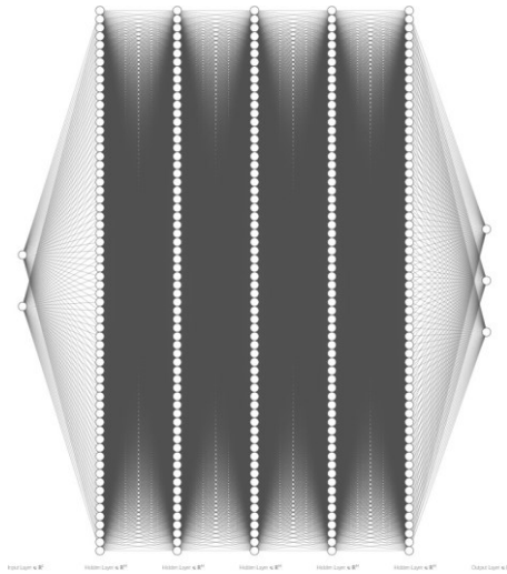
Fig.2: Neural Network schematic for the PINN, contains 2 input neurons, 5 hidden layers, each with 64 neurons each, and 1 output layer with 3 neurons. In the input layer, the spatial coordinates x and y are represented as neurons, In the next 5 hidden layers, each with 64 neurons are responsible for capturing and learning the complex relationships and features within the fluid flow data. In the output layer, the velocity components in the x and y directions are received along with the pressure.
