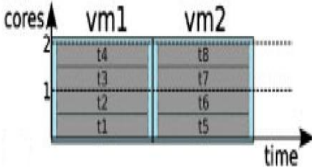
Fig. 9 Vms have Space-shared provisioning and tasks time-shared provisioning [11]
