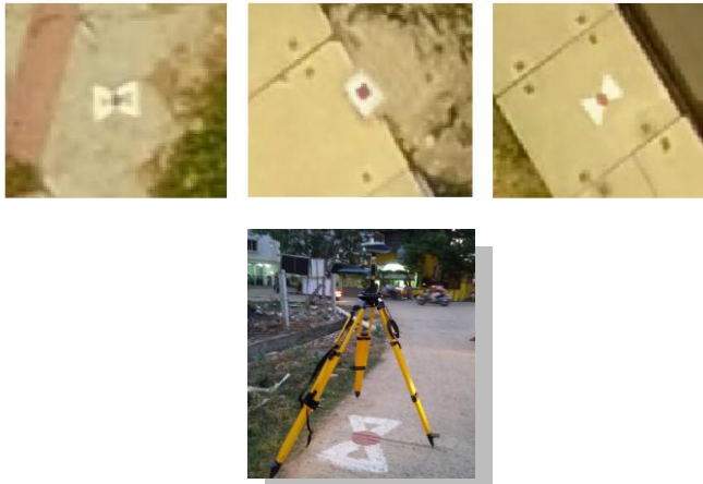
Fig-2 Sample Control Point Markings
