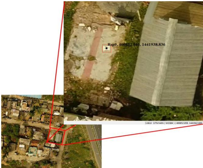
Fig-8 Control Point Overlay on Ortho Photo
