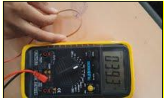
Figure 6: Snapshot of Change in Resistance with Bending of flex sensor
