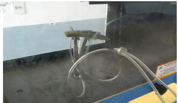
Fig (24) Pressure distribution test
