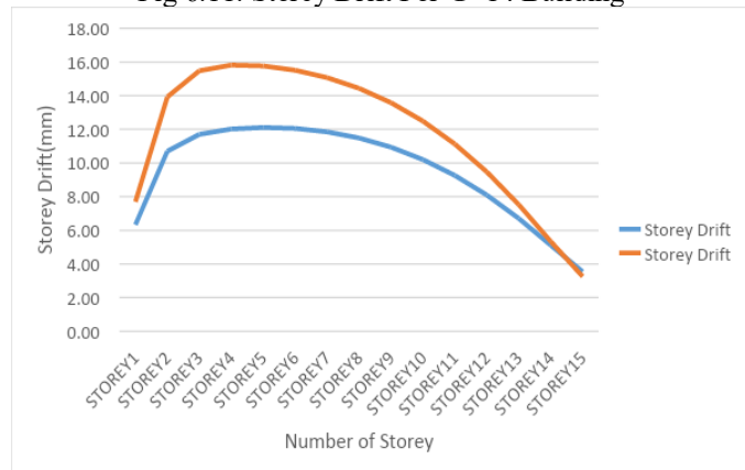
Fig 6.11: Storey Drift For G+14 Building
