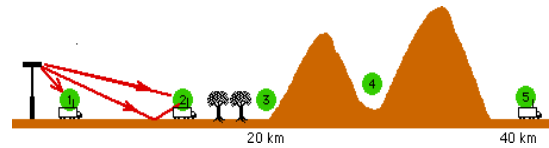
Figure 1. Path loss model depends on the location of the receiving antenna.
